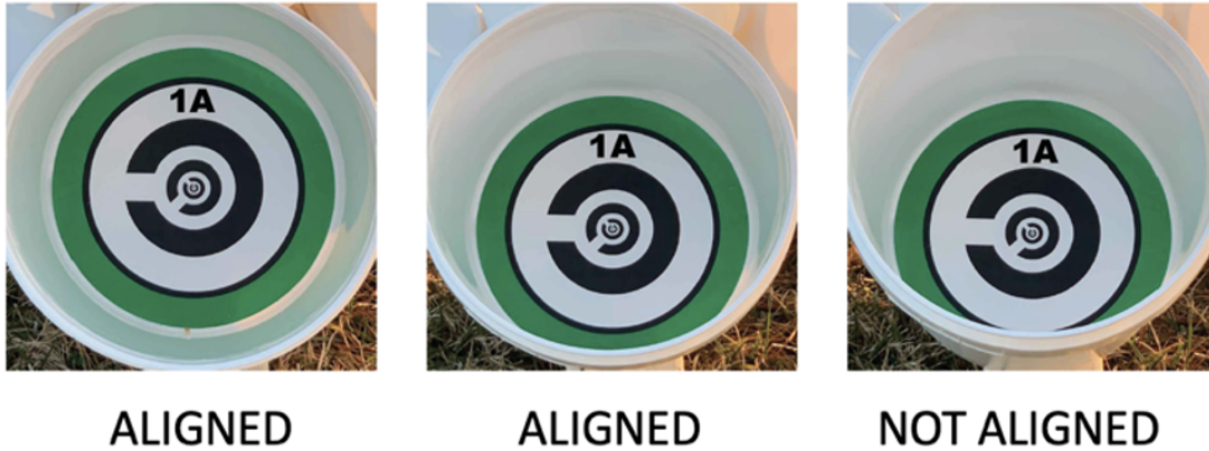
Figure 4: Correct alignment is defined as when the operator is able to see the entire black or white outer ring outside of the Landolt Cs (inside of the colored ring), as shown in the left and middle image.
