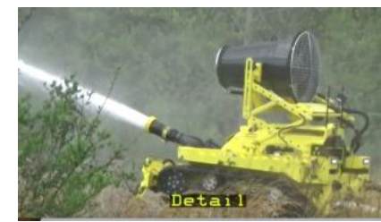
Howe & Howe Thermite RS1 & RS3 550kg (1200lbs) 1200 Gallons per Minute
