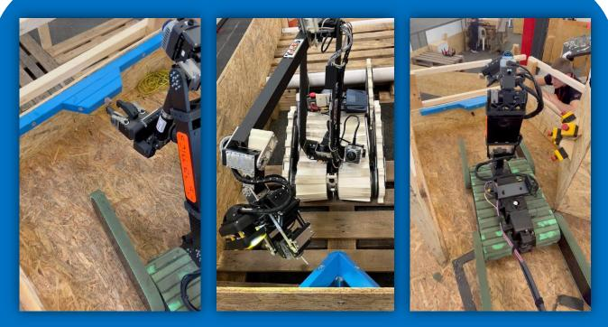
One of the standard dexterity tests is "Touch" tools which is conducted in every terrain. See the blue apparatuses shown in both Linear (easier) and Omnidirectional (harder) configurations.
