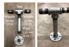
12 mm (1/2 in) PIPE-T HANDLE 1 Pipe, 2 Flanges, 1 Tee, 2 Nipples
